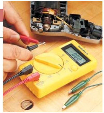
Meter Check – Touching the two probes of a multi-meter together should produce a zero reading — just like when checking for continuity.
