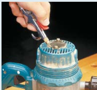
A. Remove Dust – With the tool running, blow air through the intake slots to remove packed-in dust.
